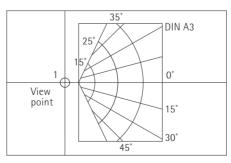
Grid for calculating the contrast rendition factor, taking as a basis an A3 format area of view at viewing position (1), 50 mm in front of and 400 mm above the front edge of the area under consideration.
