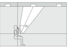
By projecting the field of vision onto the ceiling surface it is possible to define the area in which the luminaires may have a negative influence on contrast rendering. For the basic planning of a lighting installation the CRF value is generally only calculated for the primary viewing angle of 25°.
