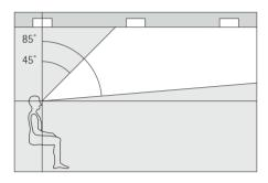
To evaluate direct glare the luminance of the luminaires within the range 45° to 85° is considered.
