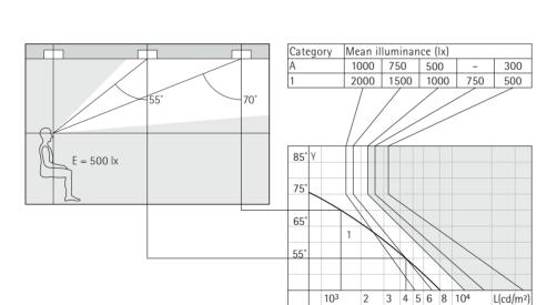
Example of how to apply glare limitation to an illuminance level of 500 lx and category A. From the geometry of the space the viewing angle for the first luminaire is 55°, for the second luminaire 70°. The corresponding luminances can be read off luminance curve 1 in the diagram.
